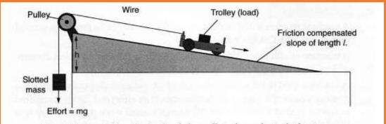
Fig. 14.9: How the length of inclined plane affects the mechanical advantage.
