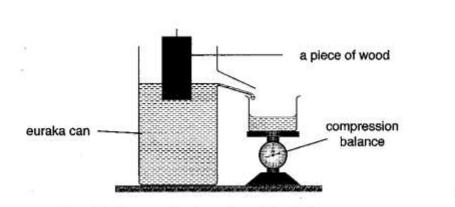
Fig. 4.1: Density of a piece of wood by displacement
