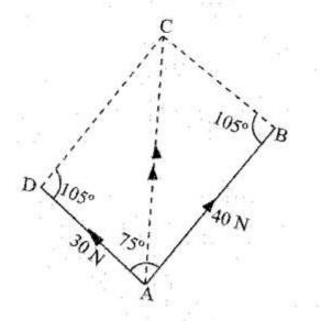
ABCD is a parallelogram AD // to BC AB // to DC angle ADC = 180° - 75 = 105° angle ABC = <ADC = 105 AC is the resultant force.
