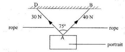
Fig. 5.11: Portrait suspended using two ropes
