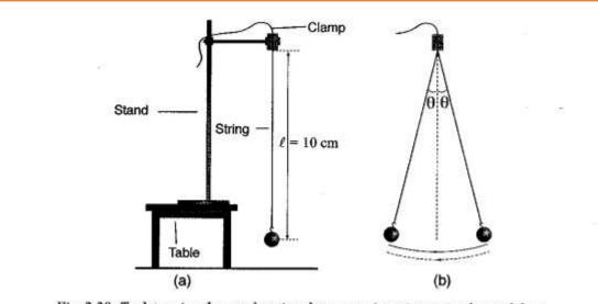
Fig. 2.28: To determine the acceleration due to gravity using a simple pendulum
