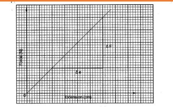
Fig. 9.2: Force-extension graph for a spring.
