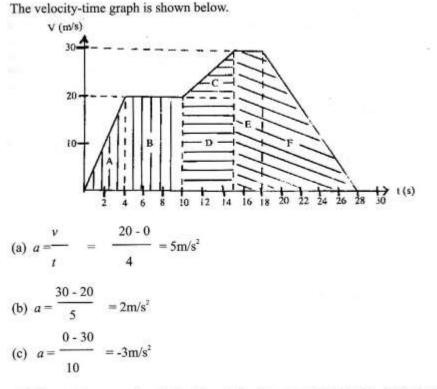
(d) The total area may be obtained by adding the areas of sections A, B, C, D, E and F which are triangles and rectangles, or the shaded areas which are trapezia. Using the latter, we get total distance = First shaded area + Second one + Third one
