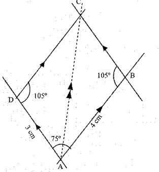
We obtain Fig. 5.13. AC is the resultant force. AC = 5.6=  $5.6 \times 10$  N = 56 N <CAD =  $44^{\circ}$
