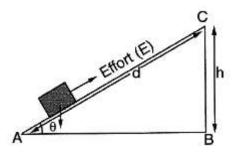
It is easier to move a heavy load from **A to C than** from **B to C**.
