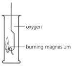
Magnesium ribbon is lit over a Bunsen flame, and plunged into a jar of oxygen. It burns with a brilliant white flame, leaving a white ash, **magnesium oxide**: Hot iron wool is plunged into a gas jar of oxygen. It glows bright orange, and throws out a shower of sparks. A black solid is left in the gas jar. It is **iron(III) oxide**:
