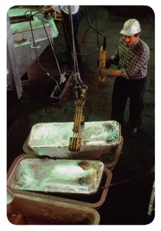
▲ Moltem aluminium from the tank was run into these moulds, to make blocks.
