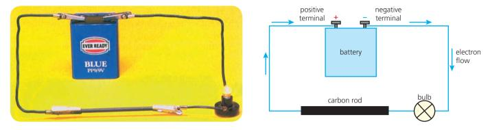
The photograph above shows a battery, a bulb and a rod of graphite joined or **connected** to each other by copper wires. (Graphite is a form of carbon.) This arrangement is called an **electric circuit**.
