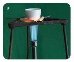
The crucible contains calcium carbonate. If you keep on heating, it will all decompose to calcium oxide and carbon dioxide.
