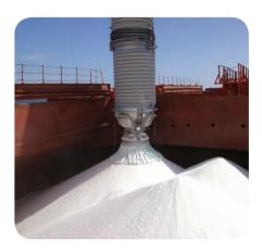
**3** The ore is taken to a bauxite plant, where impurities are removed. The result is white **aluminium oxide**, or **alumina**.
