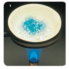
The blue crystals above are *hydrated* copper(II) sulphate. On heating, they turn to a white powder. This is *anhydrous* copper(II) sulfate: CuSO<sub>4</sub>.5H<sub>2</sub>O (*s*)  $\rightarrow$ CuSO<sub>4</sub> (*s*) + 5H<sub>2</sub>O (*l*)
