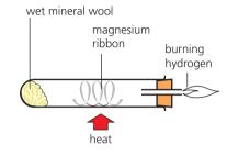
Magnesium reacts very slowly with cold water, but vigorously on heating in steam: it glows brightly. Hydrogen and solid magnesium oxide form.
