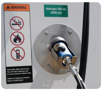
▲ Some hydrogen goes to hydrogen filling stations, for cars with hydrogen fuel cells instead of petrol engines (page 121).
