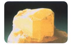
▲ This is a crystal of **rhombic** sulfur, the allotrope that is stable at room temperature.
