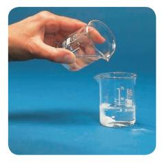
The precipitation of silver chloride, when you mix solutions of silver nitrate and sodium chloride. This is a very fast reaction.
