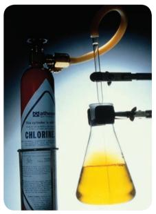
▲ Bromine being displaced by chlorine, from a colourless solution of potassium bromide. The solution goes orange.
