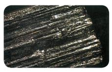
Under a microscope, you can see the layered structure of graphite quite clearly.
