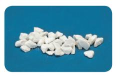
For experiment 1, large chips are used. Their surface area is the total area of exposed surface.
