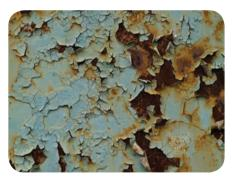
▲ Rust forms as flakes. Oxygen and moisture can get behind them - so in time the iron rusts right through.
