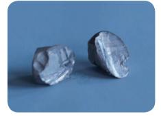
Sodium is so soft that you can cut it with a knife. It floats on water – and reacts immediately with it, forming a solution. So no good for gates. It melts at only 98 °C.
