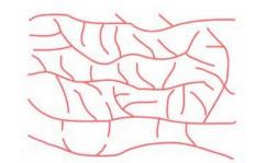
At about 200 °C, 2000 atmospheres pressure, and with a little oxygen present, the chains will branch. Now they can't pack closely, so the polythene is far less dense.
