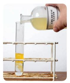
▲ Chlorine displacing bromine from aqueous potassium bromide.
