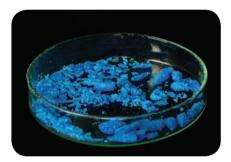
▲ Crystals of copper(II) sulfate. They are *hydrated*: they contain water molecules in the crystal structure. Their full formula is CuSO<sub>4</sub>.5H<sub>2</sub>O.
