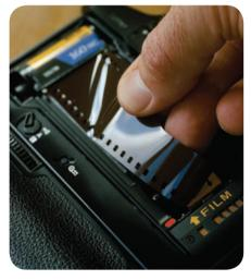
▲ Putting film in a camera. Most of the film is inside the yellow cartridge, at the top, protected from light.
