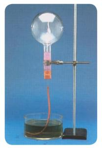
▲ The **fountain experiment**. The flask contains ammonia. It dissolves in the first drops of water that reach the top of the tube, so a fountain of water rushes up to fill the vacuum. (Any very soluble gas will show this effect.)
