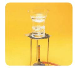
▲ Evaporating the ethanol from a solution of sugar in ethanol, over a water bath.
