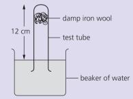
After five days the water level had risen by 2.5 cm, and the iron had rusted to iron(III) oxide.
