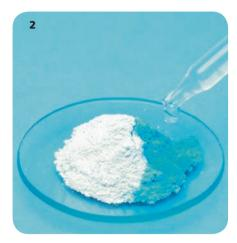
The reaction is easy to reverse: add water! The anhydrous copper(II) sulfate gets hot and turns blue. The reaction is:  $CuSO_4(s) + 5H_2O(l) \rightarrow$
