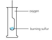
Sulfur catches fire over a Bunsen burner, and burns with a blue flame. In pure oxygen it burns even brighter. The gas **sulfur dioxide** is formed:
