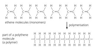
The drawing shows six ethene molecules adding together. In fact many thousands add together, giving molecules with very long chains. These very large molecules are called **macromolecules**.
