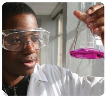
▲ You can find how much alkali is needed to neutralise acid by doing a titration using indicator, as here ...
