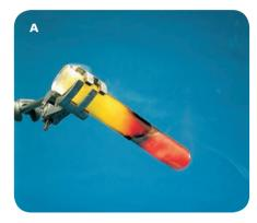
To start off the reaction between iron and sulfur, you must heat the mixture. But soon it glows red hot - without the Bunsen burner!
