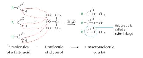
This is a **condensation reaction**, with the elimination of water. Each OH group in a glycerol molecule can react with a *different* fatty acid, so you can get many different esters. Note the ester linkage, as in Terylene (page 267).
