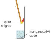
Since hydrogen peroxide breaks down very slowly, there is not enough oxygen to relight the splint. Manganese(IV) oxide makes the reaction go thousands of times faster. The splint bursts into flame.
