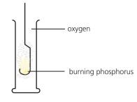
Phosphorus bursts into flame in air or oxygen, without heating. (So it is stored under water!) A white solid, **phosphorus pentoxide**, is formed:
