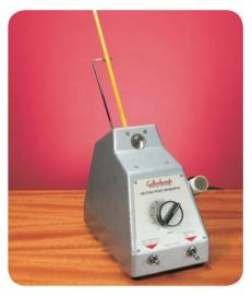
▲ Equipment for measuring melting points in the school lab. It can heat substances up to 300°C – so no good for sodium chloride!
