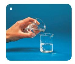
Mixing silver nitrate and sodium chloride solutions gives a white precipitate of silver chloride - and a temperature rise.
