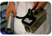
▲ Checking for radiation using a Geiger counter. The meter gives a reading, and you may also hear beeps.
