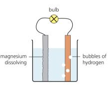
At the same time bubbles of hydrogen start to form on the copper strip, and the magnesium strip begins dissolving.
