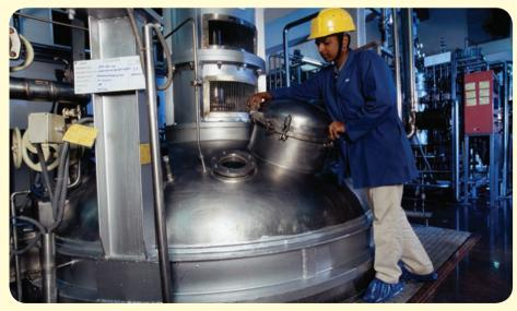
▲ Anyone home? The tank contains bacteria, busy making enzymes. For example it could be the enzyme amylase, that catalyses the conversion of starch to sugar.
