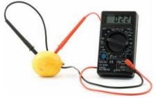
▲ The conductivity meter measures the current passing through the liquid, carried by ions. (Lemon juice contains hydrogen ions and citrate ions.)
