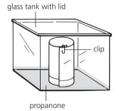
2 Stand the paper in a little propanone, in a covered glass tank. The solvent rises up the paper. When it's near the top, remove the paper.
