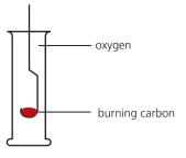
Powdered carbon is heated over a Bunsen burner until red-hot, then plunged into a jar of oxygen. It glows bright red, and the gas **carbon dioxide** is formed:
