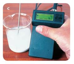
When you add water to lime (calcium oxide) heat is given out, so the temperature rises. Here the rise is being measured.
