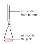
**2** Add the acid from a burette, just a little at a time. Swirl the flask carefully, to help the acid and alkali mix.
