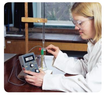
▲ ... or you could use a pH meter, to measure the pH of the solution. How will you know when neutralisation is complete?
