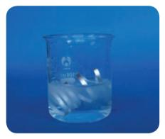
▲ Magnesium displacing hydrogen from hydrochloric acid.
