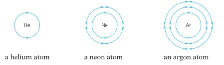
So the atoms have no need to react in order to gain or lose electrons. The noble gases are unreactive, and monatomic, because their atoms already have a stable outer electron shell.
