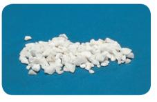
For experiment 2, the same *mass* of marble is used – but the chips are small so the surface area is greater.
