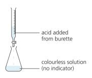
**5** Now repeat *without* the indicator. (It would be an impurity.) Put 25 cm<sup>3</sup> of alkali in the flask. Add the correct amount of acid to neutralise it.
