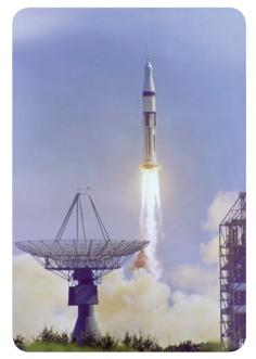
▲ The reaction between hydrogen and oxygen gives out so much energy that it is used to power rockets. The reactants are carried as liquids in the fuel tanks.
