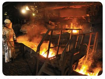
▲ Iron occurs naturally in the earth as iron(III) oxide,  $Fe_2O_3$ . This is **reduced** to iron in the blast furnace. Here, molten iron runs out from the bottom of the furnace.
