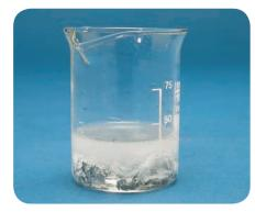
When zinc is added to dilute sulfuric acid, they react together. The zinc disappears slowly, and a gas bubbles off.
