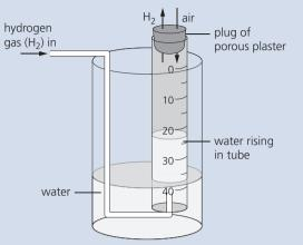
The measuring tube is sealed at the top with a plug of porous plaster. Air and other gases can diffuse in and out through the tiny holes in the plug.
