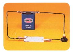
**Tin.** A strip of tin is connected into the circuit, in place of the graphite rod. The bulb lights, so tin must be a conductor.
