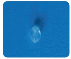
... it turns into a liquid that cools to a waxy white solid. This is found to contain very long molecules, made by the ethene molecules joining.
