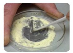
This is a **mixture** of iron powder and sulfur. You could separate them by dissolving the sulfur in methylbenzene (a solvent), and filtering the iron off.
