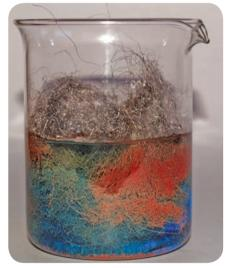
▲ Iron wool reacting with copper(II) sulfate solution. Iron is more reactive than copper so displaces the copper (deep pink) from solution.
