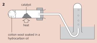
A hydrocarbon can be cracked in the lab using the apparatus above.
