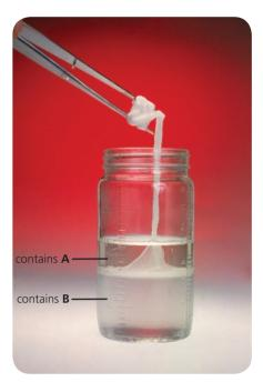
▲ Making nylon in the school lab. ▲ is dissolved in water. **B** is dissolved in an organic solvent that does not mix with water. Nylon forms where the solutions meet.
