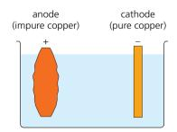
The anode is made of impure copper. The cathode is pure copper. The electrolyte is dilute copper(II) sulfate solution.
