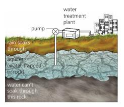
Using an aquifer as a water supply.
