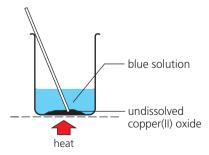
**1** Add some copper(II) oxide to dilute sulfuric acid. It dissolves on warming, and the solution turns blue. Add more until no more will dissolve ...
