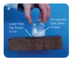
When barium hydroxide reacts with ammonium chloride, the temperature falls so sharply that water *under* the beaker will freeze!
