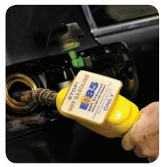
▲ Filling up with a mixture of 85% ethanol, 15% gasoline.
