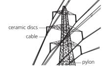
At pylons, ceramic discs support the bare cables. Since it is an insulator, the ceramic prevents the current from running down the pylon. (Dangerous!)
