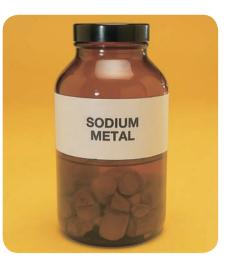
▲ Lithium, sodium, and potassium are stored under oil in the lab, to prevent reaction with oxygen and water.
