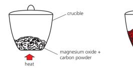
Magnesium oxide is mixed with powdered carbon and heated. No reaction! So magnesium must be more reactive than carbon. But when lead(II) oxide is used instead, it turns to molten lead, and carbon dioxide gas forms. So carbon is more reactive than lead.
