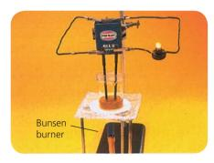
**Lead bromide.** It does not conduct when solid. But if you melt it, it conducts, and gives off a choking brown vapour.
