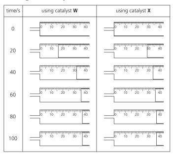
**a** Copy the table. Use the gas syringe diagrams to complete it.
