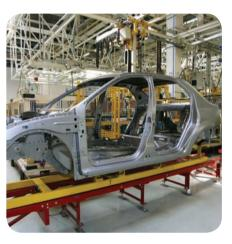
Zinc is coated onto steel car bodies, before they are painted, because zinc protects the steel from rusting, by sacrificial protection.
