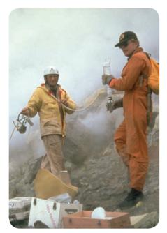
▲ Sulfur dioxide is one of the gases given out in volcanic eruptions. These scientists are collecting gas samples on the slopes of an active volcano.
