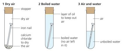
**Result** After several days, the nails in test-tubes 1 and 2 show no signs of rusting. But the nail in test-tube 3 has rust on it. This is because:
