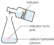
**1** Put 25 cm<sup>3</sup> of sodium hydroxide solution into a flask, using a pipette (for accuracy). Add two drops of phenolphthalein.
