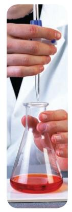
▲ The colour of the solution has changed: the titration is complete.
