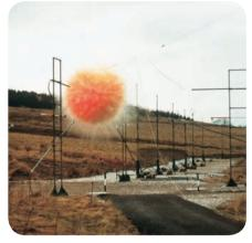
▲ Testing an explosive substance. The rate of a fast reaction like this, giving a mix of gases, is not easy to measure.
