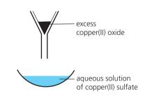
2 ... which means all the acid has now been used up. Remove the excess solid by filtering. This leaves a blue solution of copper(II) sulfate in water.
