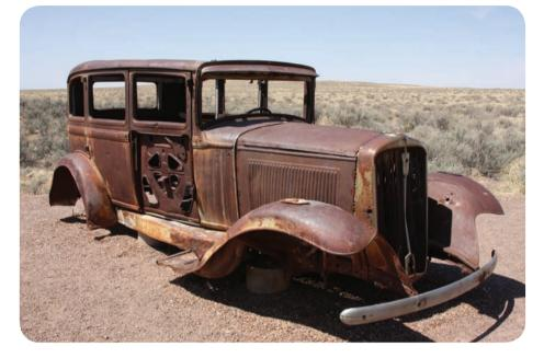
The corrosion of iron and steel has a special name: **rusting**. The red-brown substance that forms is called **rust**.
