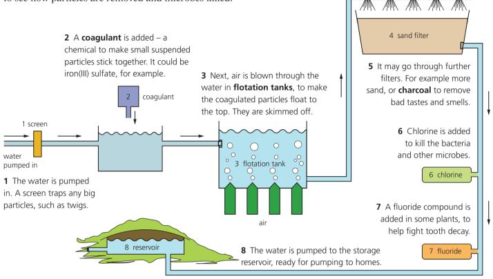
This treatment can remove even the tiniest particles. And chlorine can kill all the microbes. But the water may still have harmful substances dissolved in it. For example, nitrates from fertilisers, that can make babies ill.
