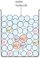
When you mix the two solutions, the barium and sulfate ions bond together. Barium sulfate forms as a precipitate.
