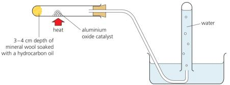
The moment heating is stopped, the delivery tube must be lifted out of the water. Otherwise water will get sucked up into the hot test-tube. Now compare the reactant and product:
