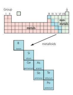
Metals conduct electricity. Metalloids can too, under certain conditions. So they are called **semi-conductors**. This leads to their use in computer chips and PV cells for solar power. Silicon is used the most.
