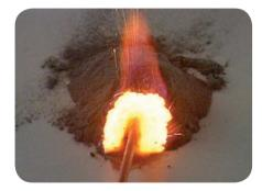
But if you heat the end of a metal rod in a Bunsen burner, and push it into the mixture, the mixture starts to glow brighly. A **chemical change** is taking place.
