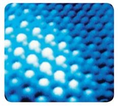
▲ This image was taken using a tunneling electron microscope. The white blobs are palladium atoms, the blue ones are carbon. (The colour was added to help us see them.)
