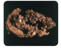
The copper crystals are called **grains**. A lump of copper like this one consists of millions of grains joined together. You need a microscope to see them.
