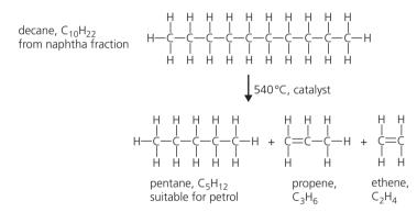
So decane has been broken down into three smaller molecules. The propene and ethene molecules have carbon–carbon double bonds. These two compounds belong to the **alkene** family, and they are very reactive.
