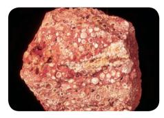
This is a piece of **bauxite**, the main ore of aluminium. It is mostly **aluminium oxide**.
