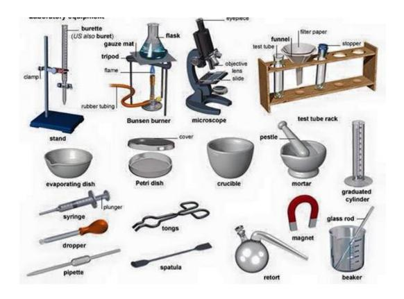
Figure; showing some common laboratory apparatus
